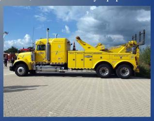
Standard tow trucks use a **wheel lift** or under-lift to pull vehicles. A wheel lift picks up the drive wheels of the vehicle (ie the front wheels if it is front wheel drive, the rear wheels if it is rear wheel drive) touching only the tires.
